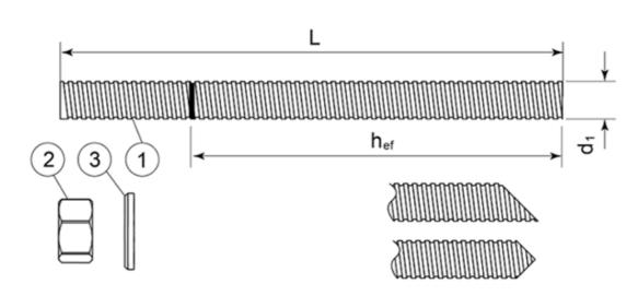
Standard commercial threaded rod with marked embedment depth
